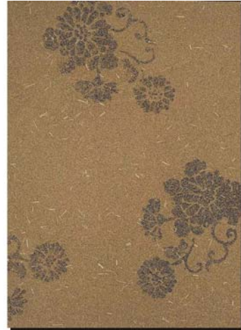
Koruku cork plaster with rice stalk fiber. Background "Cork" color. Stenciled with "Black" Koruku.
